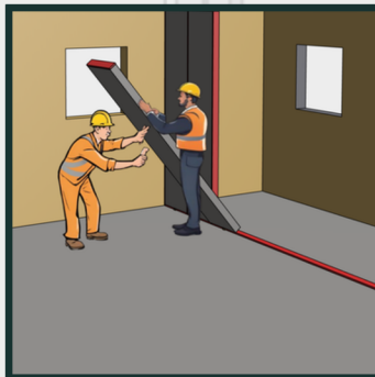
Apply bonding agent to the base alignment and sides of the PPWall, then lift the panel
